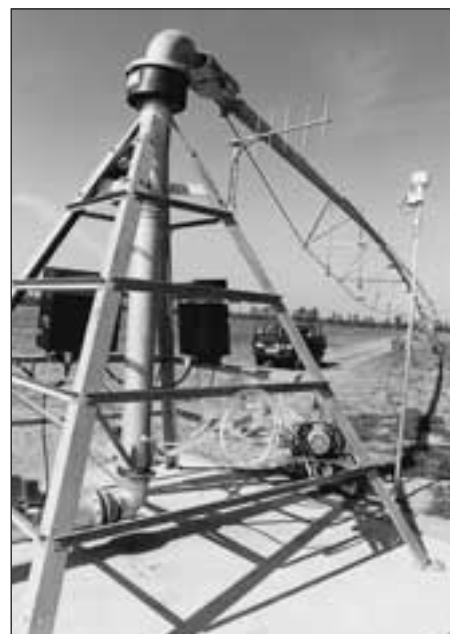
Fig. 2: Communication links at centre pivot irrigation machine
