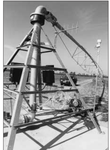
Fig. 2: Communication links at centre pivot irrigation machine
