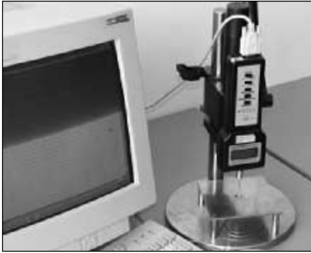
Fig. 2: Digital penetrometer for determining resistance of cooked potato slices
