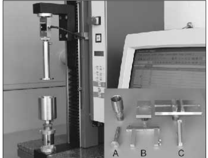
Fig. 3: Material testing machine with tools for determining the extrusion force (A), cut force (B) and fraction force (C)
