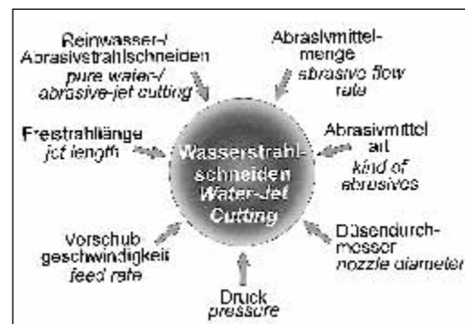
Fig. 2: Parameters of a water-jet cutting system
