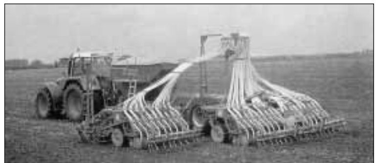
High area performance packer coulter drill from BBG-Amazon with up to 9 m working width
