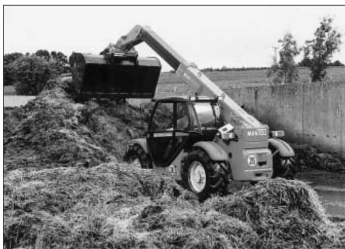
Fig. 1: Turning of solid manure improves even rotting (Photo Manitou)
