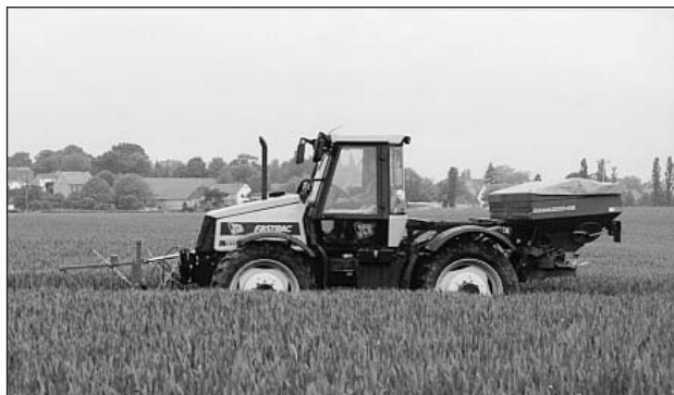
Fig. 1: Tool carrier with pendulum-meter for plant mass mapping
