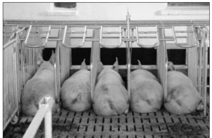
Fig. 1: Combi-feeder with opened rear door
