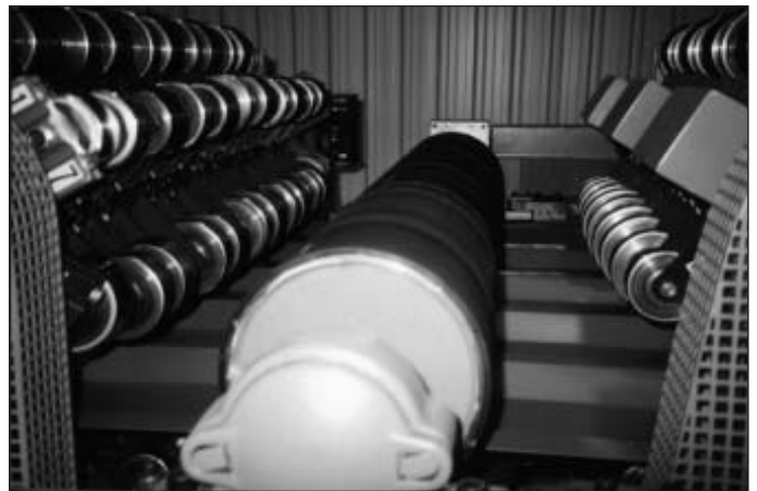
Fig. 1: Machine for producing trapezoidal corrugated sheets (Photo: Laukien Comp., Kiel)
