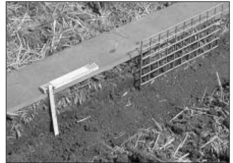
Fig. 3: Classifying with a lattice screen
