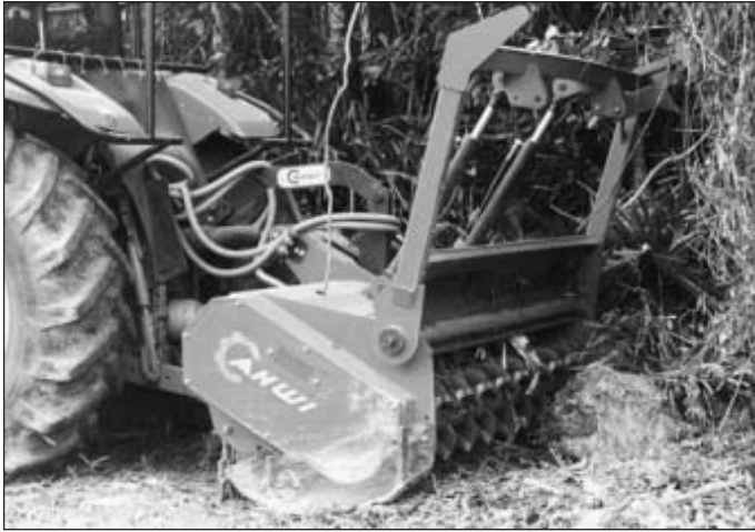
Fig. 2: Mulching machine (AHWI FM 600) working in an eight year old fallow vegetation
