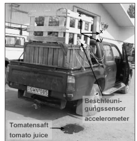
Fig. 1: Pick-up car with container half filled with tomatoes and above them with onions (16 bags each with 25 kg) to simulate the bulk height of a real truck
