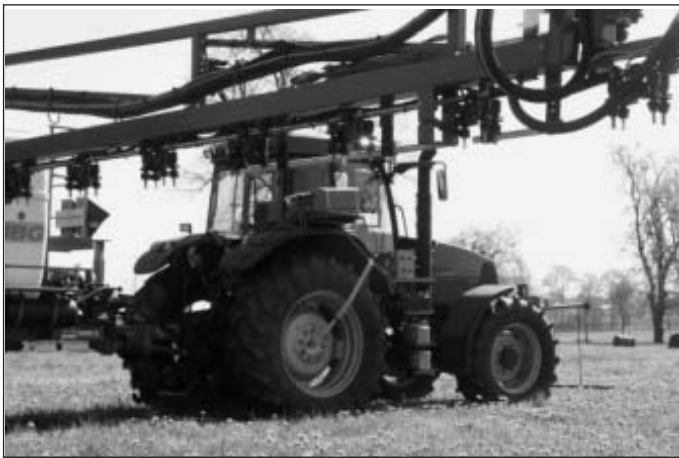
Fig. 2: Prototype of the pulled field sprayer with unfolded 24 m boom and the VarioSelect® nozzle system
