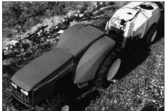
Fig. 3: Driverless GPS-controlled viticultural tractor (photo: John Deere)
