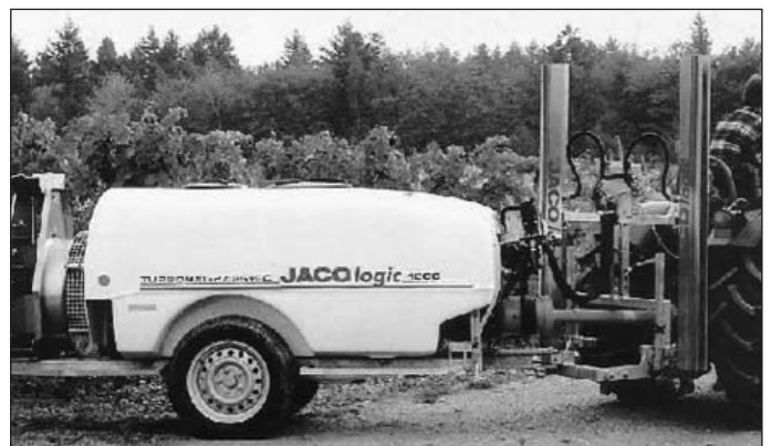
Fig. 1: Atomizer with detection of misses (photo: Jacobi)
