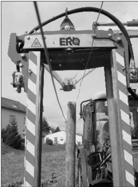
Fig. 2: Leaf cutter guided along a live trellis wire (photo: ERO)
