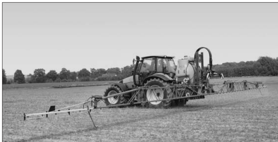
Fig. 2: Small, low gravity centre containers are characteristic for modern mounted field sprayers. Here you see the new UF 01 by Amazone with 1800 l capacity and a working width up to 28 m. Foto Amazone
