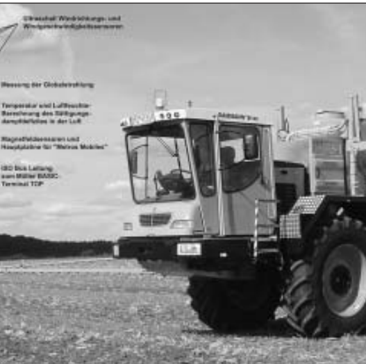
Fig. 1: With its drift optimising system „Meteos AOS“ Dammann want to achieve considerable improvement in the application of plant protectives Foto Dammann
