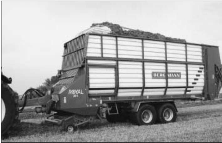
Fig. 2: A modern self-loading forage wagon with 2-rotor loading technology and a capacity of 48 m 3
