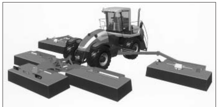
Fig. 1: Claas presents a SP-mower, too, with a working width of more than 14 m. Foto Claas
