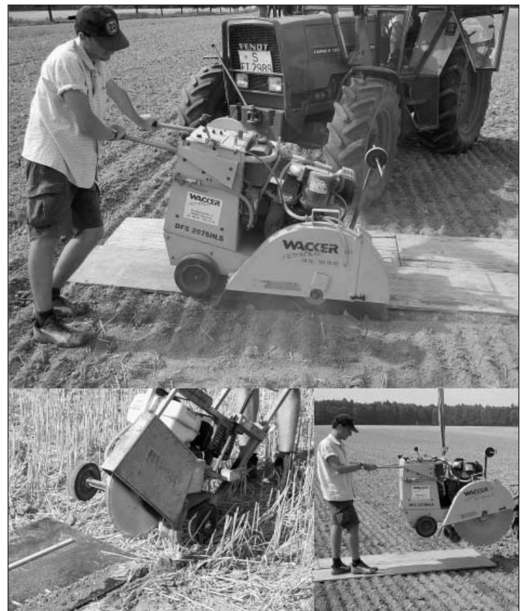
Fig. 1: Large and small asphalt floor saw for different working depths
