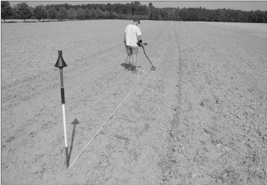
Fig. 2: Determination of the placement depth of the objects of measurement with the metal detector
