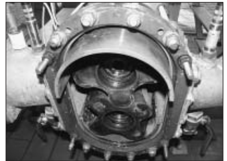
Fig. 1: Changeable insert liners of pump housing
