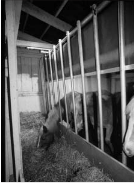
Fig. 2: Rolling feed rack with timing controlled curtain
