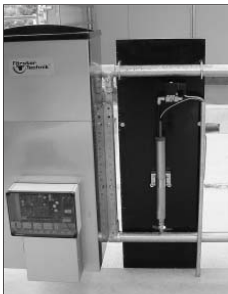
Fig. 2: Measuring cylinder of the automatic drinking water measuring system (ATS) by Förster Technik
