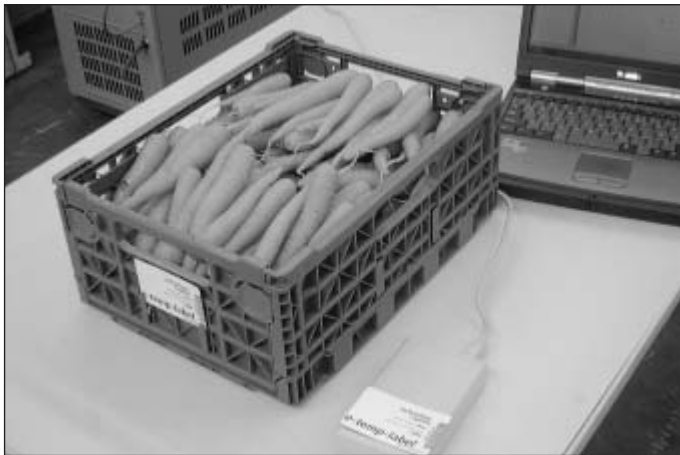
Fig. 2: Transponder card, write/read unit and host computer in operation with temperature control of carrots
