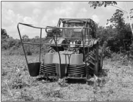
Fig. 1: Version 2.0 of the wood chopper prototype „Tritucap“
