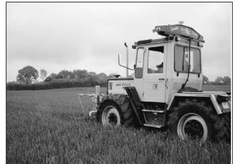
Fig. 1: Pendulum-sensor and N-Sensor on a tractor
