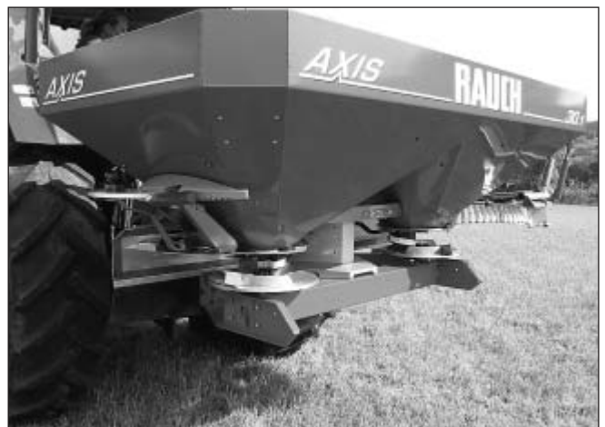
Fig. 4: The new Axis ® fertilizer spreader from Rauch with CDA spreading technology allows for high working speeds of up to 20 km/h even at large working widths and high application rates.
