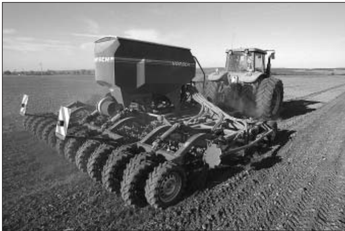
Fig. 2: With the Sprinter ST (working width: 4 or 6 m), Horsch completes the lower range of its mulch drill programme (company photo).
