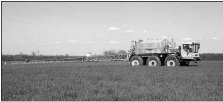
Fig. 1: Efficiency through size ñ the Dammann-trac DT 2600 H 3A with a container volume of 10,000 litres
