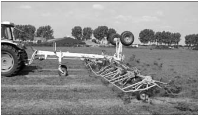
Fig. 2: The Volto 1320 T from Claas has ten rotors each with six tine stars and has a working width of 13 m
