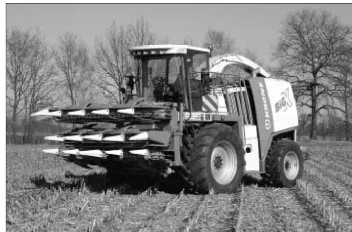
Fig. 3: The strongest Krone forage harvester Big X 1000 (here with a row-independent maize header in transport position) has two 6-cylinder in-line engines, which are connected by a synchromesh transmission on the crankshafts and provide a rated power of about 730 kW/1,000 hp
