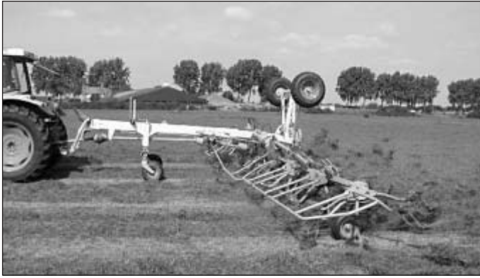
Fig. 2: The Volto 1320 T from Claas has 10 rotors with 6 tine arms each and reaches a working width of 13 m
