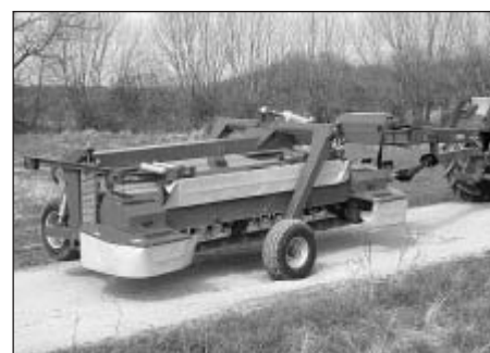
Fig. 1: At a working width of 9.2 m, the trailed disc mower GMS 4802 from JF-Stoll, which has a mowing width of 4.6 m, deposits a 2.8 m double swath. In the transport position, it is 3 m wide
