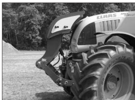
Fig. 3: The variable front weight (here on the Ares), which Claas also offers for tractor models from other manufacturers, is a smart solution
