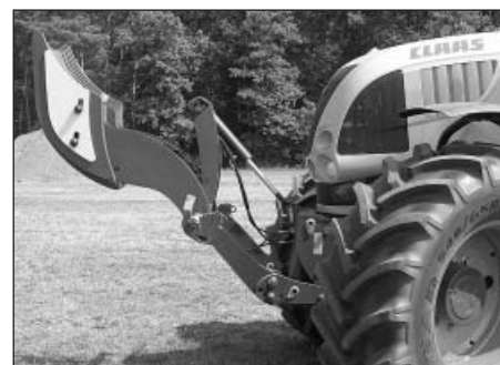
Fig. 3: The variable front weight (here on the Ares), which Claas also offers for tractor models from other manufacturers, is a smart solution
