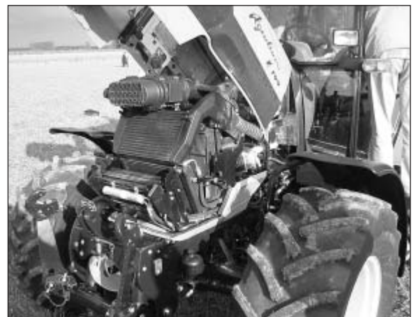
Fig. 1: The cooling systems of tractors are becoming more and more sophisticated in order to optimize capacity, mounting space, and exhaust emission reduction. Here, the cooling system of the new Agrottron K 100 is shown (photo: Dr. Metzner)
