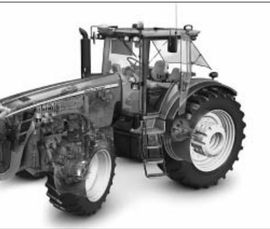
Fig. 2: The new 8030 tractors from John Deere consume 5% less fuel despite more power. They conform with exhaust emission stage IIIA and produce 40% less NO 2 .
