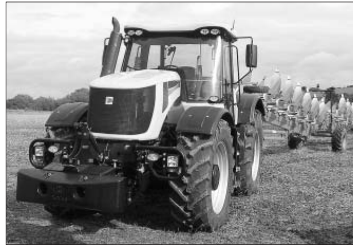
Fig. 4: JCB is travelling new avenues with its 185 kW Fastrac 8250, which has a maximum speed of 65 km/h and a modified Vario transmission
