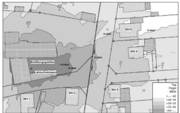
Fig. 1 and 2: Grid computation with presentation of iso-areas for the ranges: < 45 dB(A), 50 dB(A), 55 dB(A) and > 60 dB(A). The noise source is a grain ventilation fan with a fictitious sound capacity level of 105 dB(A) during day time. The images show the noise distribution in the vicinity of the plant in a height of 5.60 m. In Fig. 2 (at right) a noise protection wall is erected around the aggregate, which allows to meet the day threshold value of 60 dB(A) for the village area within the range of nearby residential quarters.
