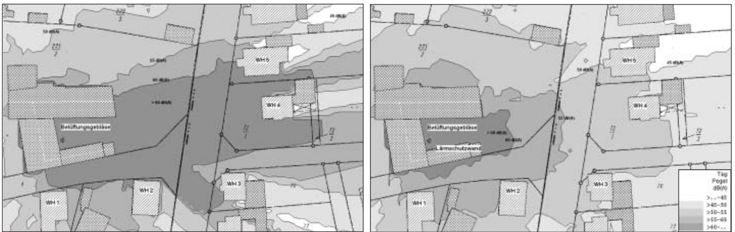
Fig. 1 and 2: Raster calculation with marked iso-areas for the ranges < 45 dB(A), 50 dB(A), 55 dB(A), and > 60 dB(A). The source of sounds is a grain ventilation fan having a fictional sound power level of 105 dB(A). The duration of operation corresponds to the period of evaluation (during the day). The figures show noise distribution in the surroundings of the facility at a height of 5.60 m. In Figure 2 (right), the unit is surrounded by a noise protection wall, which allows the daytime standard value of 60 dB(A) for the village area to be kept in the zone near residential areas.
