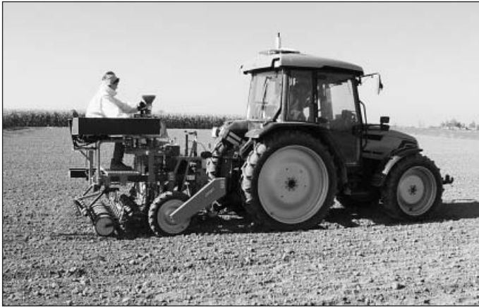
Fig. 1: Tractor with plot drill during automated seeding
