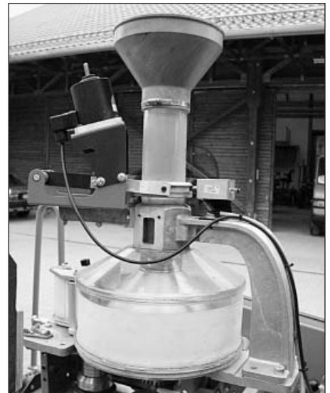
Fig. 2: Seed hopper with lifting magnet
