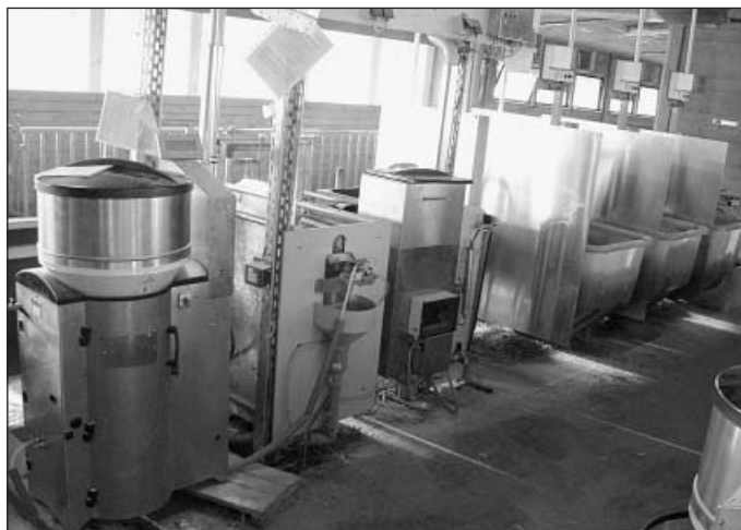
Fig. 1: System set-up (from left to right) milk feeding robot, feeding station with temperature measuring system and animal weighing system, concentrate feeding robot, drinking water robot and separated roughage weighing troughs
