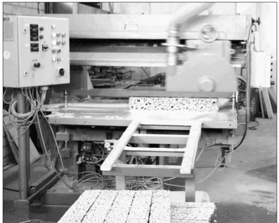
Fig. 3: Cutting of stalk core blocks with a plate chop saw
