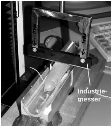
Fig. 2: Cutting equipment for carrots with industrial knife by using a universal testing machine
