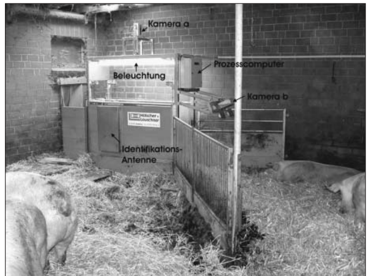
Fig. 1: The image processing system for automatic health supervision by Hölscher+Leuschner for sows in group housing was awarded with a gold medal.
