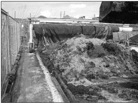
Fig. 2: Clamp digester with unwinding device (source: Hans Wolfertstetter)
