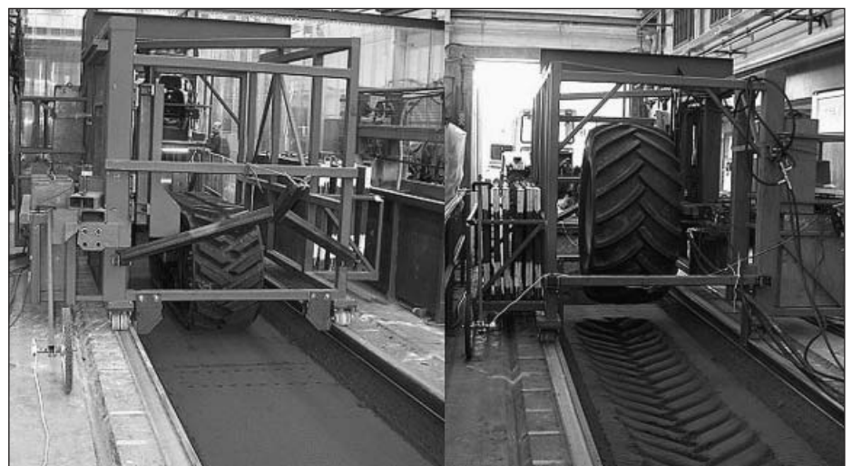
Fig. 1: Single Wheel/Track tester with a track (left hand side) before and a tire (right hand side) after a run
