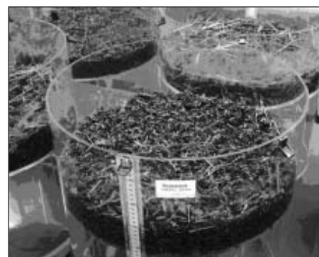
Fig. 1: Experimental container with a mixture of short-chopped wheat straw and layer hen droppings
