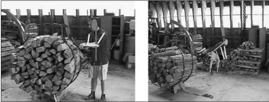
Fig. 2: Examples of code allocation for body postures according to OWAS; example 1 (left): code 1111; example 2 (right): code 2151
