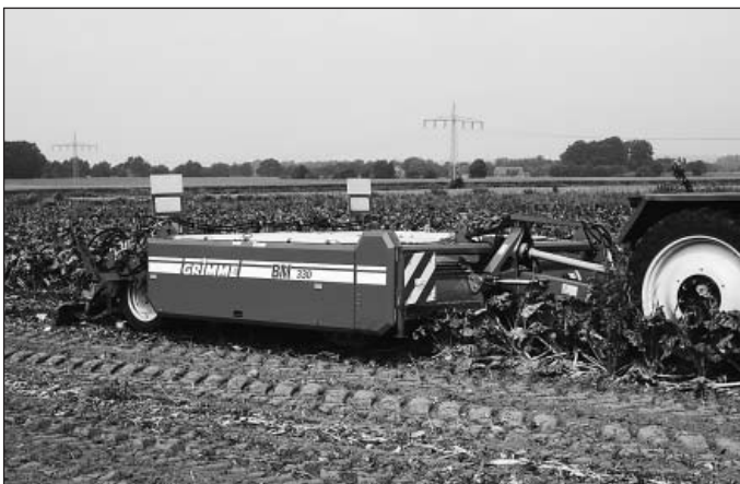
Fig. 3 and 4: Reduced to the minimum: The drawn high-capacity beet-top mulcher BM330 (left) and the 6-row drawn beet harvester Rootster 604 with a 4-t overloading hopper from Grimme, which were specially developed for the conditions in Eastern Europe
