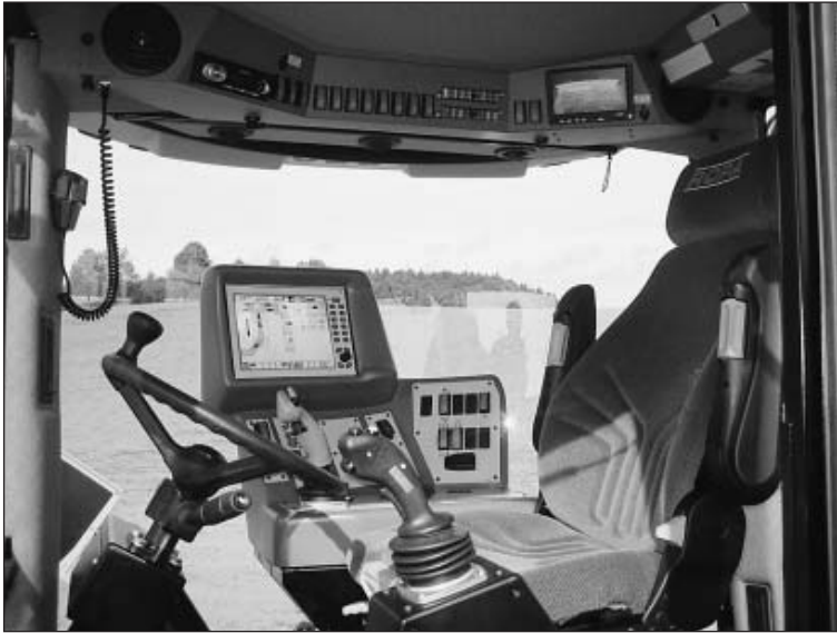
Fig. 2: View of the cabin of the new euro-Maus 3 fro, Ropa with a large, clearly-structured terminal
