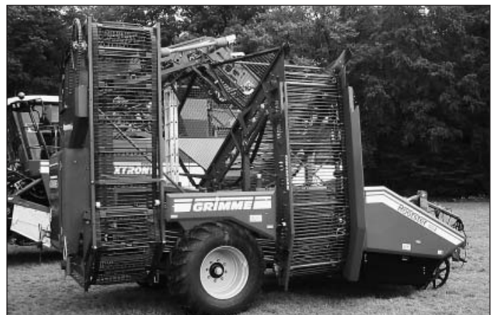
Fig. 3 and 4: Reduced to the minimum: The drawn high-capacity beet-top mulcher BM330 (left) and the 6-row drawn beet harvester Rootster 604 with a 4-t overloading hopper from Grimme, which were specially developed for the conditions in Eastern Europe
