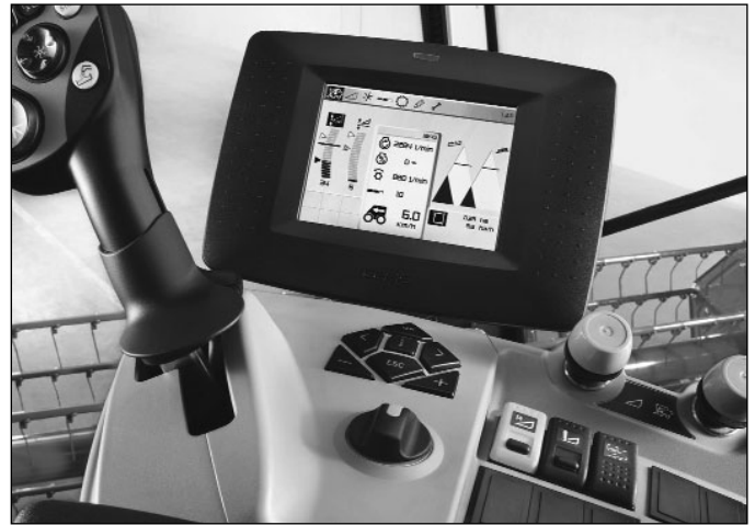
Fig. 2: Claas display and control unit for combine harvester Tucano (courtesy of Claas)
