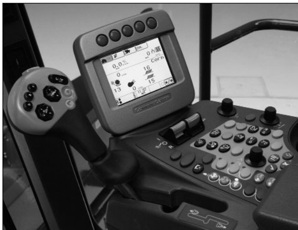
Fig. 1: John Deere display and control unit for combine harvester S690i (courtesy of John Deere)
