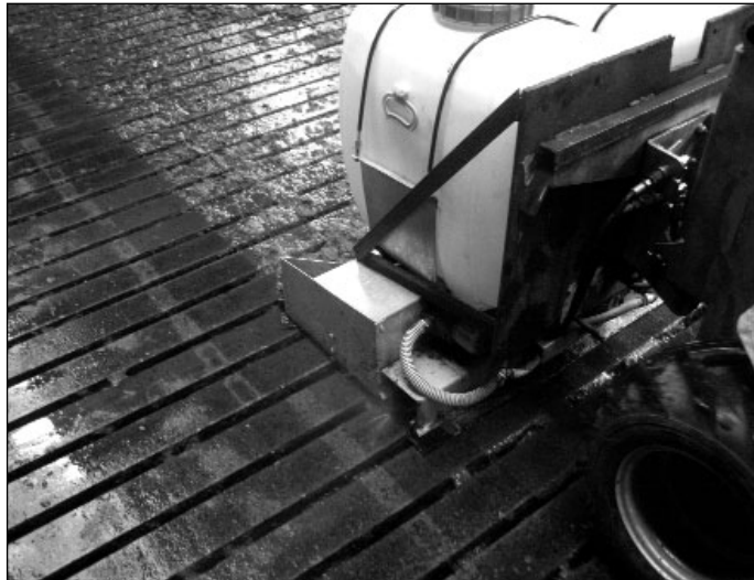
Fig. 2: With the Cleanmeleon 3 (gold medal winner) Westermann presents a modular slat cleaner which effectively cleans both surfaces and interstices. (Gold medal)
