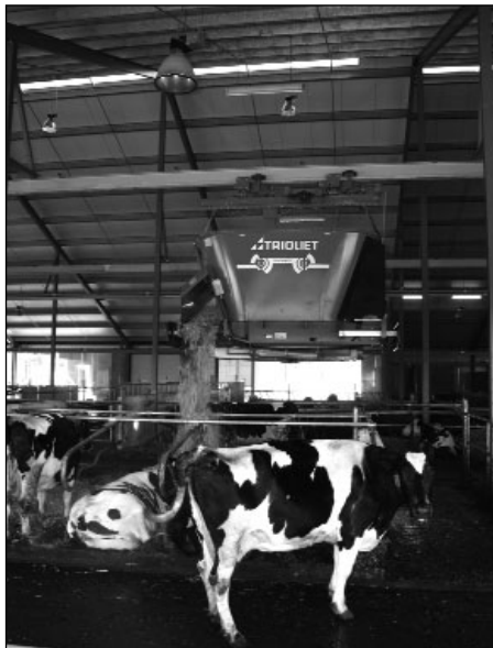
Fig. 1: Fully automatic spreading of litter is carried out by the Triomatic-System from Trioliet. Company photograph
