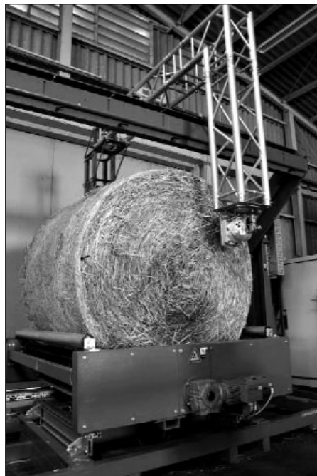
Fig. 3: The test stand measuring a round bale in the laboratory
