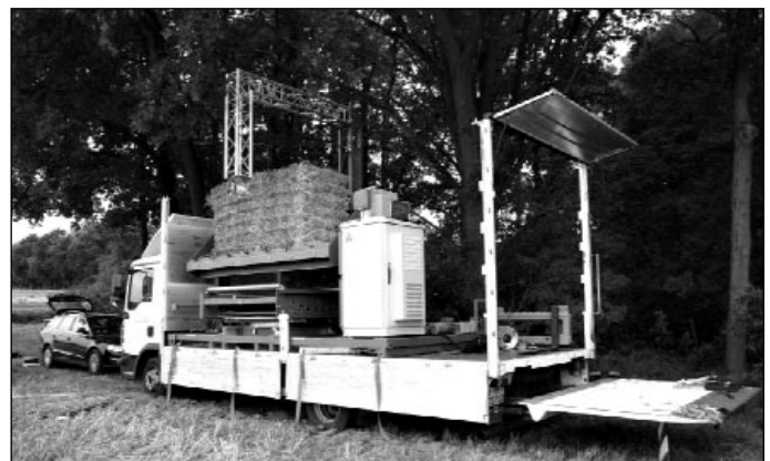
Fig. 2: The mobile test stand on a 7.5 t lorry while measuring a square bale in the field
