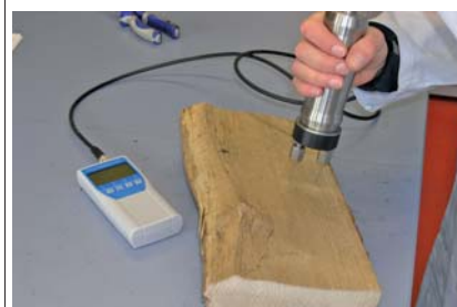
Test device using the electrical conductivity via ram electrodes
