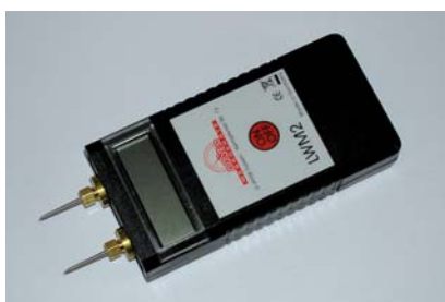
Test device using the electrical conductivity via steel needles
