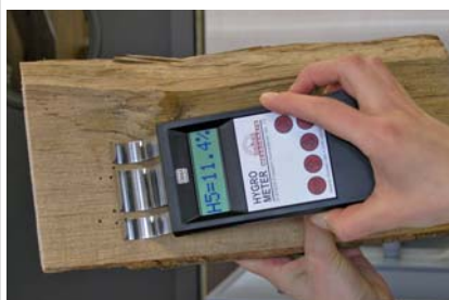
Test device using the dielectrical principle
