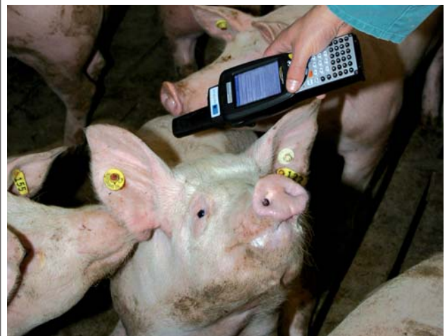
Mobile management application by using a PDA with RFID Reader as example
