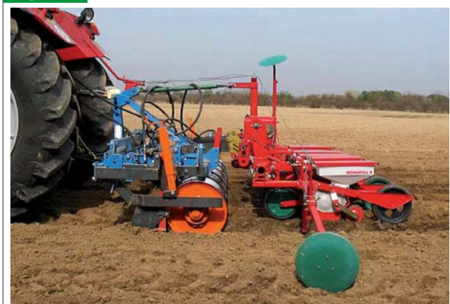
Ridge cultivator of the Department for Agriculture Engineering Bonn with Kverneland precision seeder Monopil S. Photo: Roller
