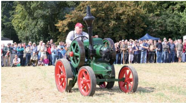
Lanz Bulldog HL 12, from 1923, built as selfpropelled heavy-oil engine
