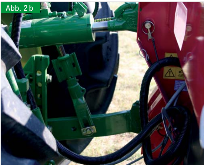
Fig. 2 b: Clearance between tractor and fertilizer spreader
