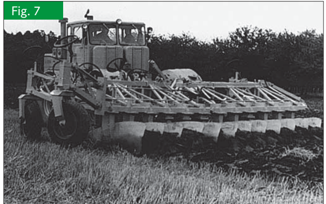
Experimental-plough with frame joints (working width B = 6 m; staggering distance S = 13,5 cm) [5]
