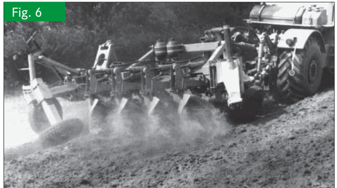
Short-plough (working width B = 2,0 m; staggering distance S = 18 cm)
